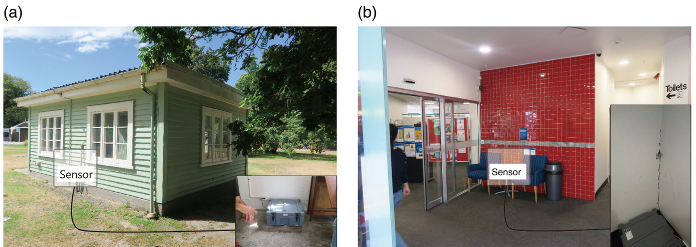
Figure 10. Installation conditions at (a) CDBG and (b) SHLC. Sensor positions are indicated. The color version of this figure is available only in the
